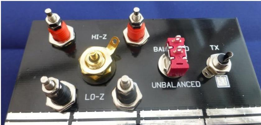
There is nothing awkward about mounting most of these components - please make sure that the lipped insulating washer that is part of the gold phono connector is fitted into the hole properly from the socket side of the panel. This insulates the outer of the socket from the earthed PCB. You will need to bend the tag on the TX socket outer so it is easier to solder to.
